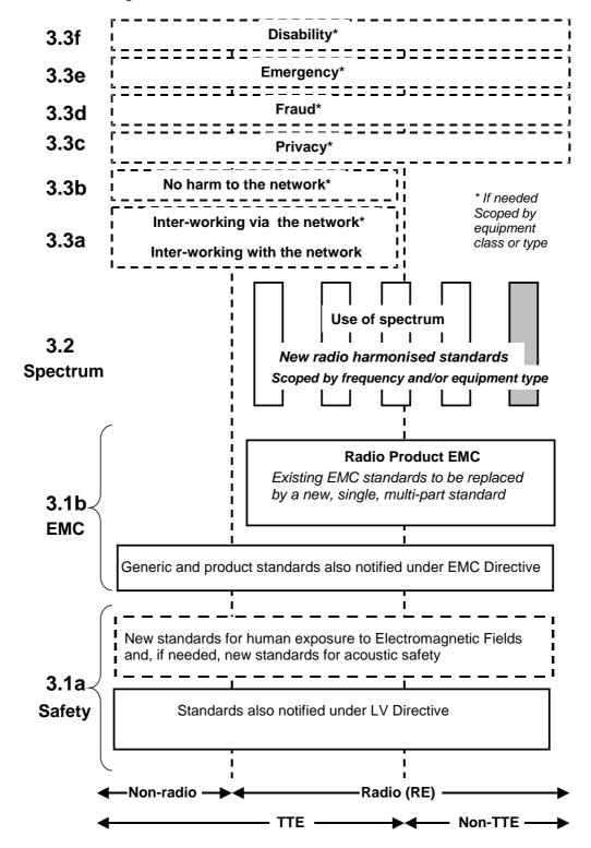
Figure 1: Modular structure for the various standards used under the R&TTE Directive [1]
