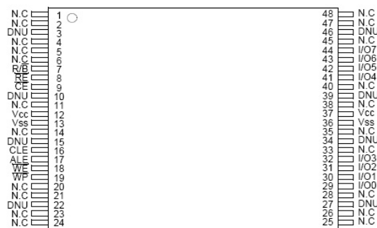
Fig. 2. Typical electrical interface of a NAND flash chip
